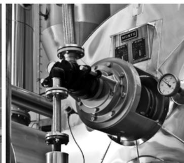
**The batch cooker is a pressure vessel with a heated jacket.** The steam heated rotor assures uniform mixing, heating, sterilization and drying of the raw material. The rotor is driven mainly by a hollow shaft gearbox. The unit can be supplied completely with cyclone, steam house, fittings and safety valves, steam ramp and condensate trap system, insulation, load cells and frame or customized.
